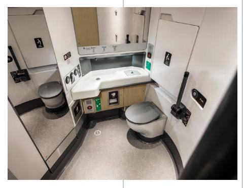
of the population. Fortuitously for those designing trains, much of this guidance is clearly defined and measurable (*e.g.* toilet door controls shall be between 800-1200m above floor level). Elements of the design that are objectively defined in this manner can be readily assessed using drawings and CAD models.
