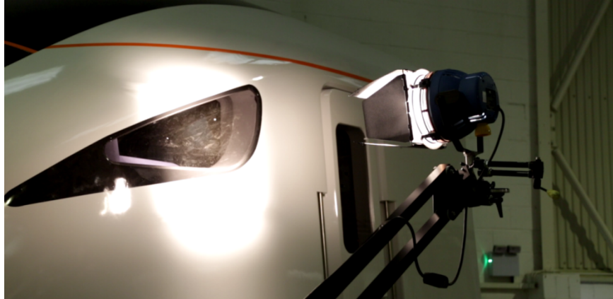
Figure 4: Arrilite light source on a Hague CamCrane K16DV aligned to one of the positions on the train side window
